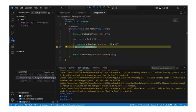
GUI applications will show up on the display defined in the settings.json. This can also be a virtual display using RDP, see chapter 7.1 for more informations.
